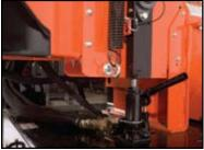
Built-in hydraulic jack makes feed roller maintenacnce quick and easy.
